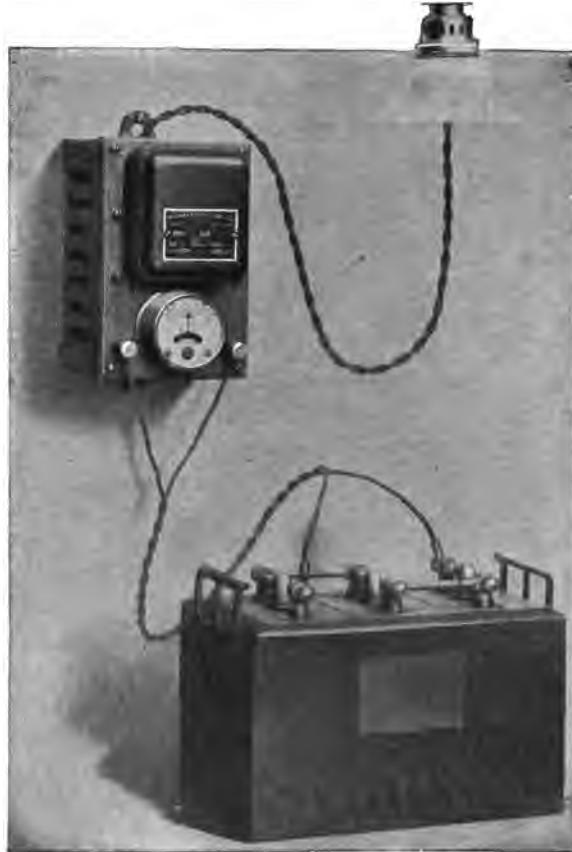
FIG. 75.—Wagner rectifier-charging storage battery.
